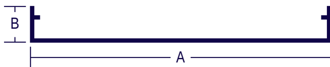
Sign Frame - No Retainer
