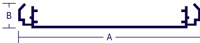
Sign Frame - No Retainer
